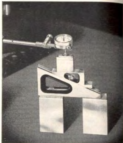
With Gage Blocks for Setting Up Work on a Surface Plate
